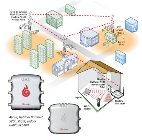
Wi-Fi access to any indoor or outdoor location without the need for backhaul cabling. HotPoint access points can also connect directly to a conventional wired infrastructure eliminating the need to install a mesh node in locations where wired connectivity is readily available.
